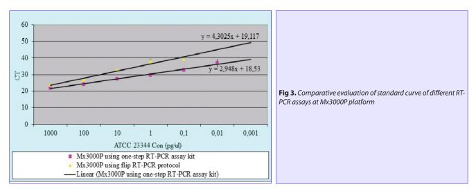
analytical sensitivity of one-step RT-PCR with Mx3000P, lower limit of detection (LOD) for *B. mallei* ATCC 23344<sup>T</sup> purified DNA was determined to be 10 fg, corresponding to 2 genome equivalents. However, *fliP* RT-PCR using Mx3000P platform determined LOD of 100 fg, 10 genome equivalents) (*Fig. 3*).
