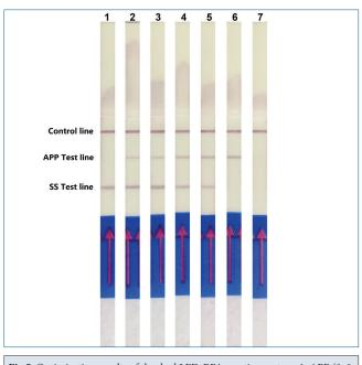
**Fig 5.** Optimization results of the dual LFD-RPA reaction system. 1. APP (0, 0, 0), SS (2, 2, 0.6). 2. APP (2, 2, 0.6), SS (2, 2, 0.6). 3. APP (2, 2, 0.6), SS (1.5, 1.5, 0.45). 4. APP (2, 2, 0.6), SS (1, 1, 0.3). 5. APP (2, 2, 0.6), SS (0.5, 0.5, 0.15). 6. APP (2, 2, 0.6), SS (0, 0, 0). unit (μL). 7. negative control
