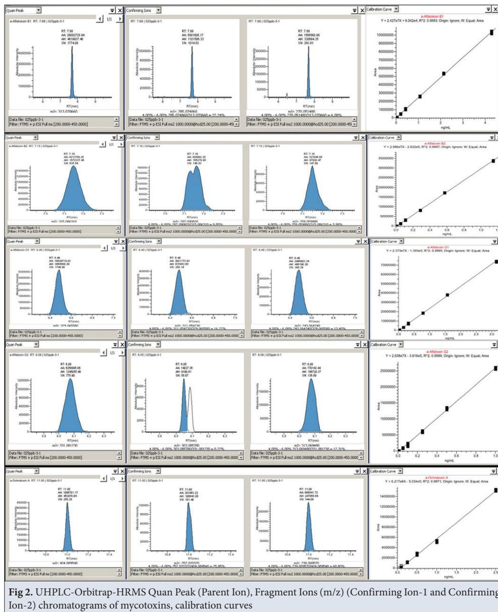
Fig 2. UHPLC-Orbitrap-HRMS Quan Peak (Parent Ion), Fragment Ions (m/z) (Confirming Ion-1 and Confirming Ion-2) chromatograms of mycotoxins, calibration curves
